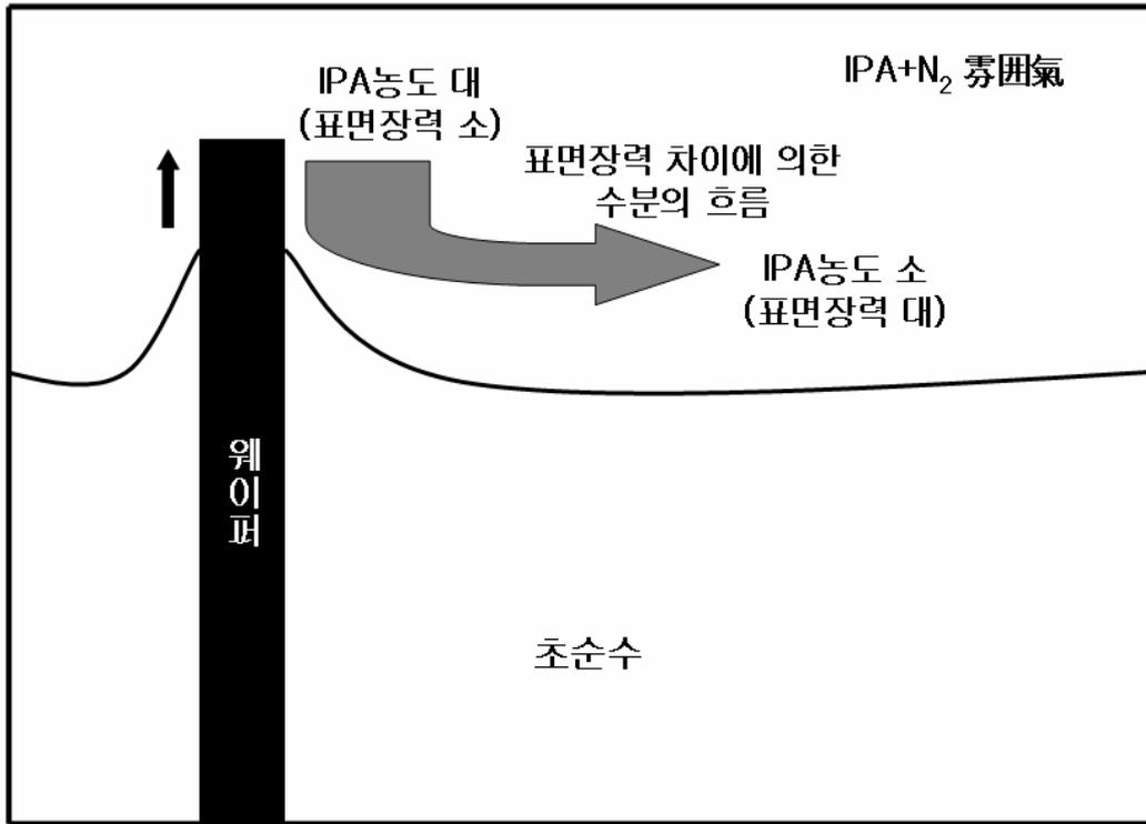
1. water-mark-less (Water-mark-less Drying)
